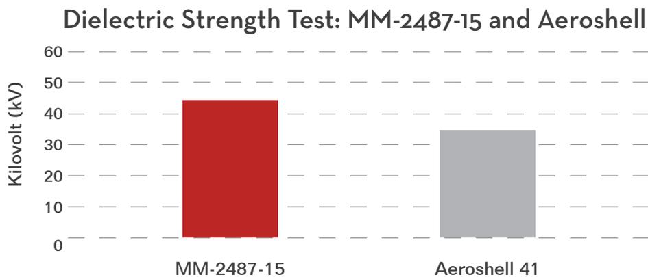
Figure 3. Dielectric Strength Test for MM-2487-15 and Aeroshell 41
