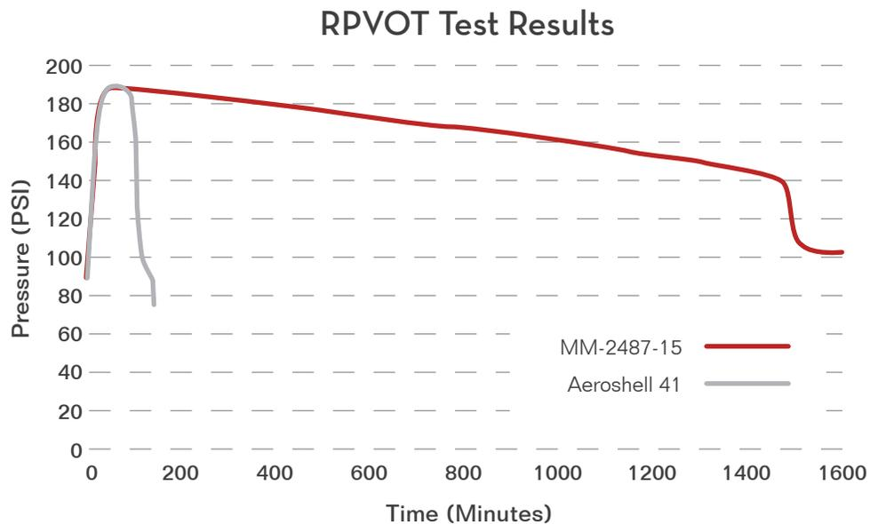
Figure 2 RPVOT Profile Comparison Chart for MM-2487-15 and Aeroshell 41
