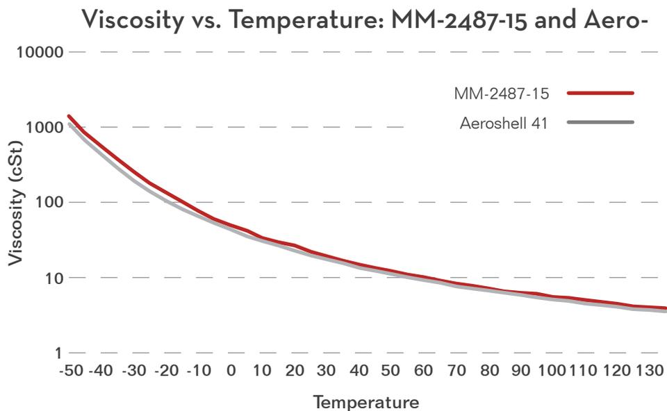
Figure 1. Viscosity vs. Temperature Profile for MM-2487-15 and Aeroshell 41 [-50 to 135°C]
