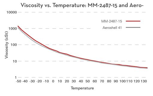
Figure 1. Viscosity vs. Temperature Profile for MM-2487-15 and Aeroshell 41 [-50 to 135°C]
