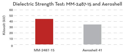
Figure 3. Dielectric Strength Test for MM-2487-15 and Aeroshell 41
