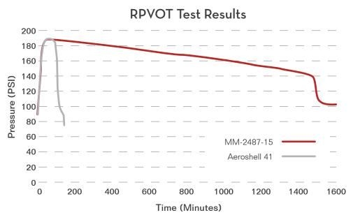
Figure 2 RPVOT Profile Comparison Chart for MM-2487-15 and Aeroshell 41
